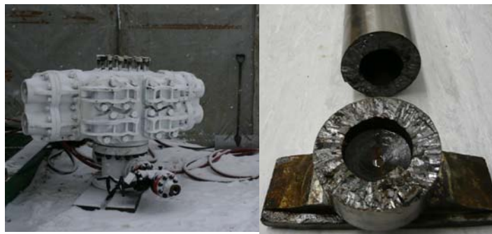
The cause of the BOP problem encountered in week 6 was a broken pipe ram
