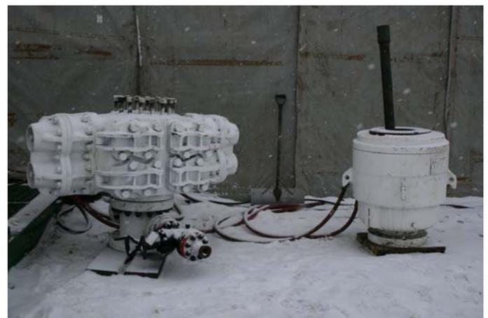
*The Achilles heel of week 6- The BOP components prior to rigging up. The annular on the right and the rams on the left are mounted on the well casing one on top of the other. Both function to provide isolation from the well pressures down hole. Both must function to conduct well operations.*
