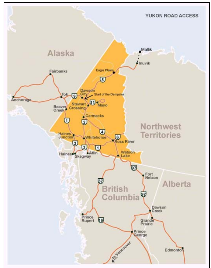
3240 km logistics route via Alberta, BC, Yukon, NWT highway system to Inuvik and 190 km ice road to Mallik
