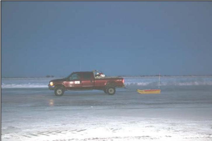
Ground probing radar is towed behind a Grubens truck to profile ice thickness before moving heavy loads to Mallik. While the ice was generally >1 m for most of the channel and sea ice areas, there was a short section with only 70 cm of ice.
