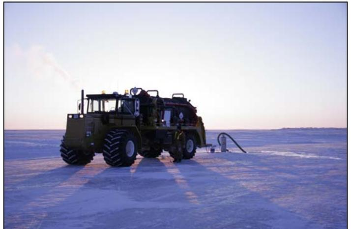
All terrain vehicle called a Gator working to spread water on lease.
