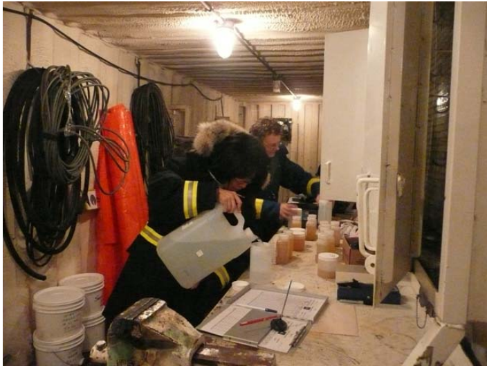
Kasumi and Fred-san working on water samples collected during testing. Lab testing will determine the change in water and gas chemistry vs. time and also quantify the grain size of the sediment retained in the sand screens.
